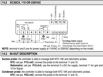
Ratiometric: set par. P2C=0-5; use the terminal 9 (+5V) for supply, terminal 11 for gnd and 10 for Signal Thermostat input: use terminals 14-17. HP input: use terminals 15-17. DLT PTC 990ohm sensor: set P3C=dLt, then connect the probe to terminals 16-17. CPA connection: not available. Power supply: use terminals 4-5. Compressor: use terminals 1-3. FAN 1: use terminals 6-7 (only for XC30CX).
