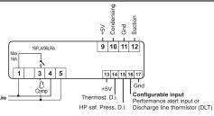
NOTE: terminal 4 and 5 are for power supply at 110VAC or 230VAC depending on the model.
